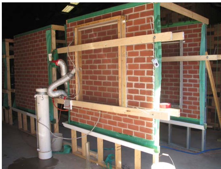
Figure 1; E514 Test Chamber on Wood Stud Sample Wall (foreground) and Metal Stud Wall (behind)
